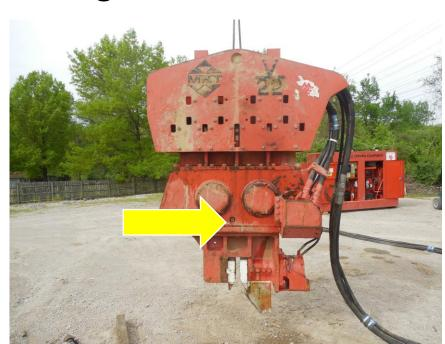
Lube oil level should be ½ to ¾ full. Check oil level twice per day.
