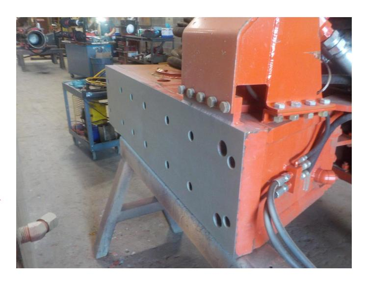
Install line up pins in proper threaded holes to align the clamp in the center of the MKT V-22 Vibratory hammer.
