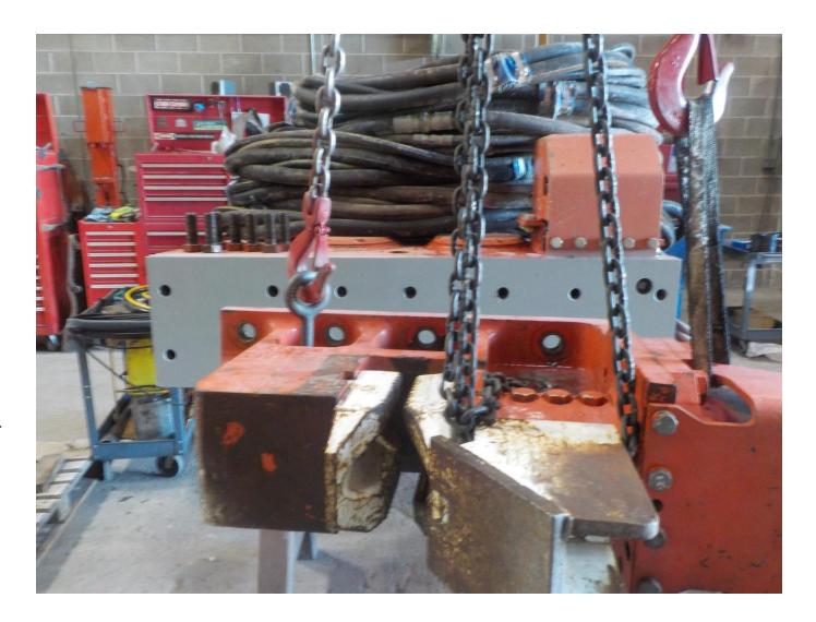
With Line up pins in place and the Clamp suspended, slowly swing the Clamp onto the line up pins. Make sure that you center the Clamp on the MKT V-22 Vibratory Hammer.
