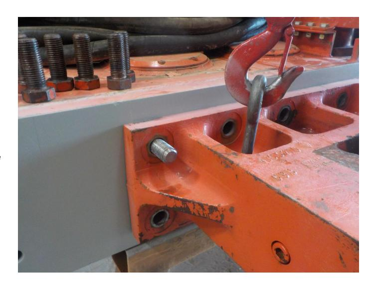
Apply a liberal coating of Anti-Seize Lubricant to the  $1 \frac{1}{2} \times 6 \times 4$  bolts. You will only need to apply it to the first 2 inches of threads.
