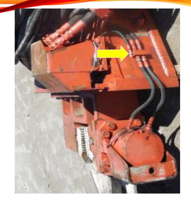
When ever the hydraulic lines of the MKT V-22 system have been reconnected and or when hydraulic repairs have been made, the clamp cylinders must be bled of entrained air.
