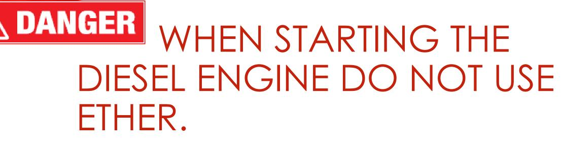
The engine is equipped with an electric heater starting aid and the use of ether may cause severe injury.
