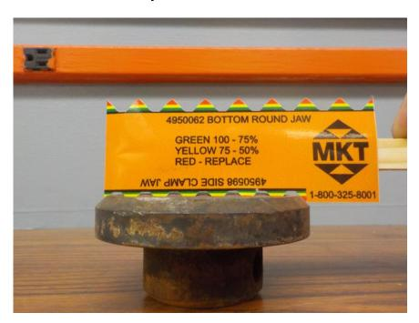
As you can see the red is not visible and the jaw reaches the yellow portion of the gauge. This indicates the jaw is still in the 75% to 50% range.
