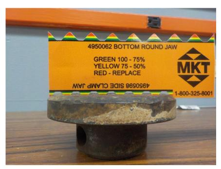
As you can see the red is visible and the jaw is beyond the 50% wear. This jaw is recommended to be replaced.
