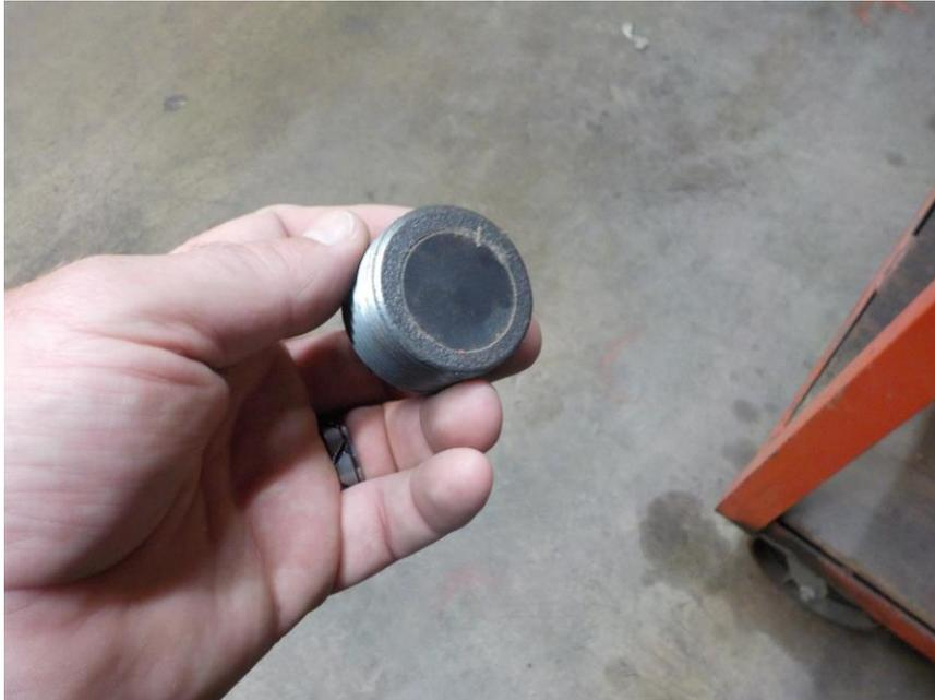
Apply a thread sealant to the pipe threads on the drain plug. This can be liquid Teflon or Teflon tape.
