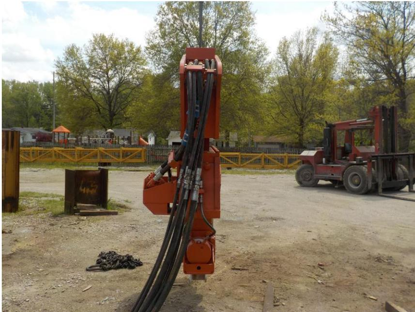
Remove the fill plug to vent the case before draining the oil. Use 18 inch crescent wrench for this step
